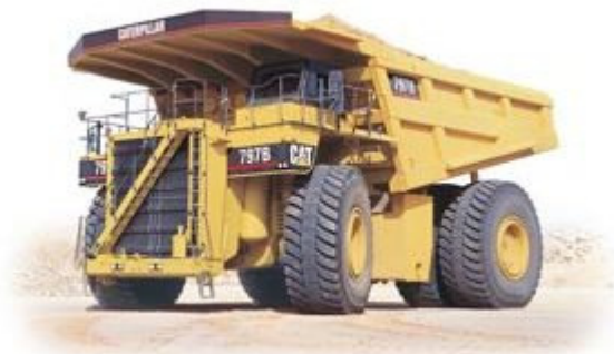
The 797B Mining Truck carries up to 380 tons
